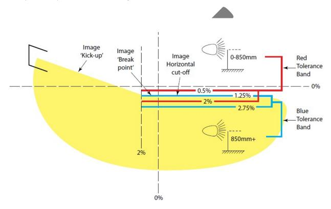
Check on dipped beam and determine that:
